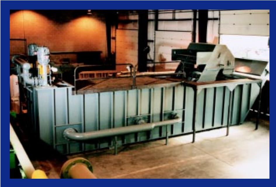
Endless belt continuous filtration with the option of disposable media
