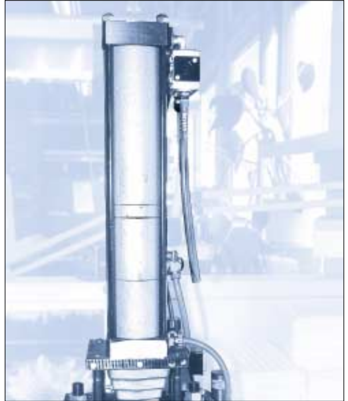
The picture above shows a pneumatic press where hose silencers have effectively eliminated impulse noise.
