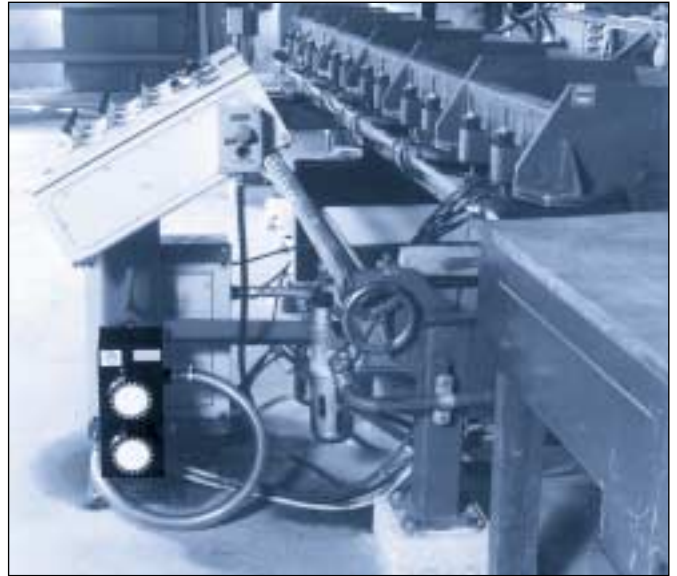
Here, an OPUS ED 1023 is connected to a folding machine with 2 x 7 rubber bellows.
