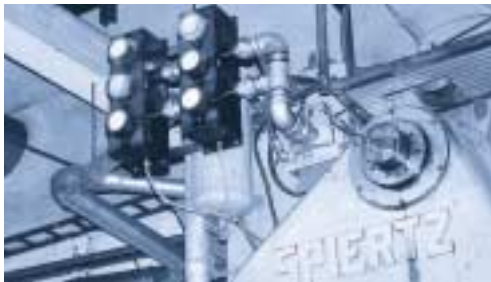
SKF has used two ED2033s to solve a noise problem in a powder press. By serially connecting the silencers they got the expansion volume they needed to avoid backpressure in the system.
