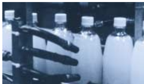
Coca Cola uses SILVENT nozzles to dry bottles before applying labels.
