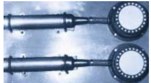
The picture shows two central silencers connected in parallel in an Italian bottle-making machine. Installing a CD lowered the noise level of the exhaust air an incredible 30 dB(A).
