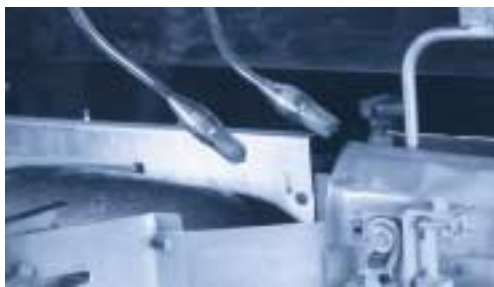
Here SILVENT 200 nozzles inflate a plastic bag, allowing bread to be packaged automatically.
