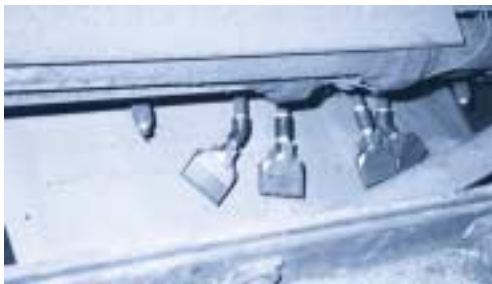
Nippon Steel in Japan uses SILVENT's stainless steel 973 flat nozzles to both clean and dry steel plate.
