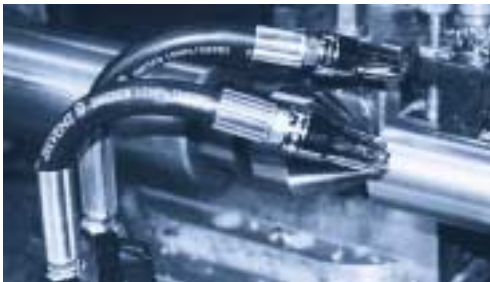
A SILVENT 232 with a magnetic base is used for blow-off when turning piston rods. The magnetic base combined with a Flexblow hose allows easy adjustment to the most efficient and quietest blowing angle.
