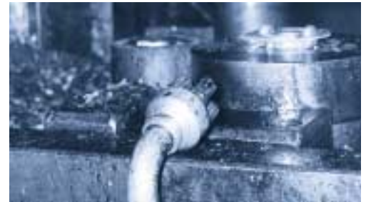
This application where parts are ejected from a press resulted in the noise level being reduced by more than 50% when a SILVENT 404 was installed.
