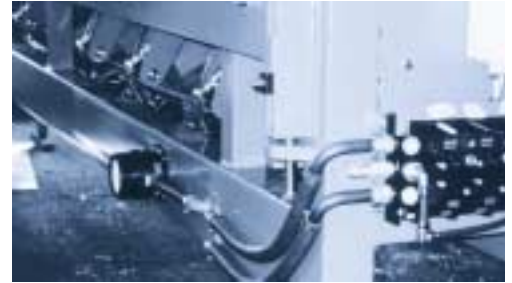
The picture shows a part of a CATECH 540 edge optimizer unit ready for delivery to Carter Holt Harvey, KOPU sawmill in New Zealand. Particularly large dimensions of the pine "Pinus radiata" are sawed in New Zealand. The picture also shows how the exhaust ports of several valves are connected to a single SILVENT central silencer.
