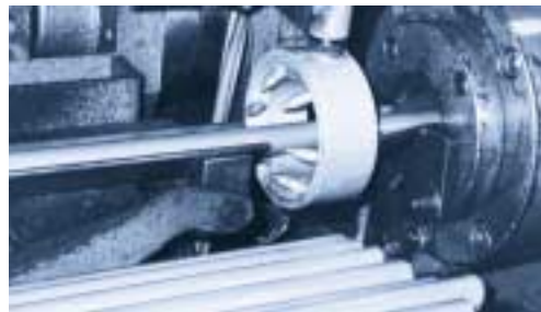
SILVENT's 456 doughnut nozzle automatically blows every pipe clean as it passes through the nozzle during production.
