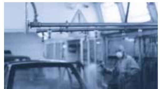
SILVENT 208s are used at Ford in Germany for drying after leak testing.
