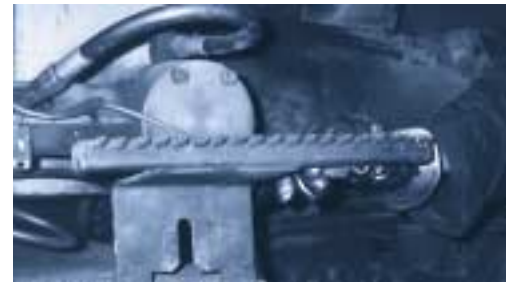
One of the largest wheel rim manufactures in Europe, Prins Dokkum in Holland, uses SILVENT air nozzles in a number of different blowing operations. The picture shows a manifold fitted with SILVENT 511 nozzles. The manifold is used to blow off scale and dirt after spot welding.
