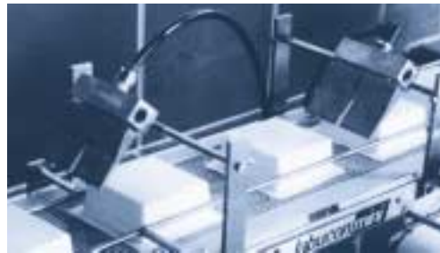
The picture shows a conveyor for cheese packaging. SILVENT 392 air knives dry the packages before labeling.
