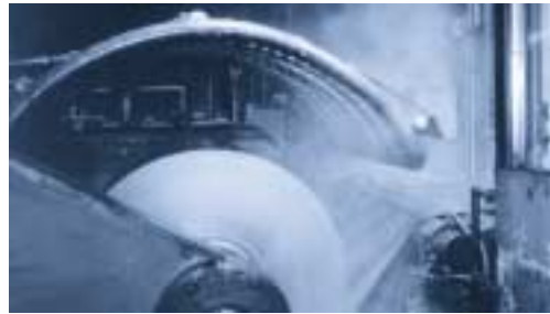
The picture shows the final phase of the sheet metal production process with SILVENT 920s. The nozzles dry the metal effectively, thereby preventing oxidation that lowers the quality of the steel.
