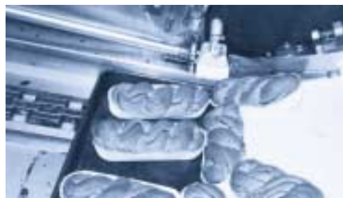
Yamazaki Bread, with more than 40 bakeries throughout Japan, uses SILVENT's stainless steel 973 F flat nozzles with adjustable flow regulation. The nozzles are used both to transport loaves of bread along their conveyors and to remove bread from the pans. Flow regulation allows easy adjustment of the blowing force required to transport and separate different sized loaves.
