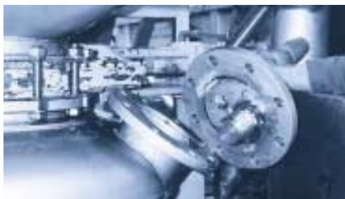
In this application SILVENT's stainless steel 720 nozzle is used to blow a filleting machine free of fish scraps. The 720 replaced an open pipe that generated a noise level of 102 dB(A). The noise level dropped to 79 dB(A) after the installation while the blowing force was more than sufficient.
