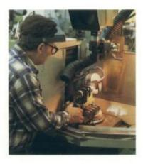
Exact geometries are ground on PCD tools with our sophisticated tool grinders.
