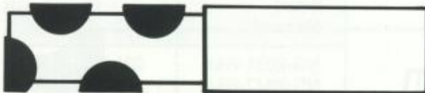
Staggered Cut Special design used for cutting edges longer than 1".
